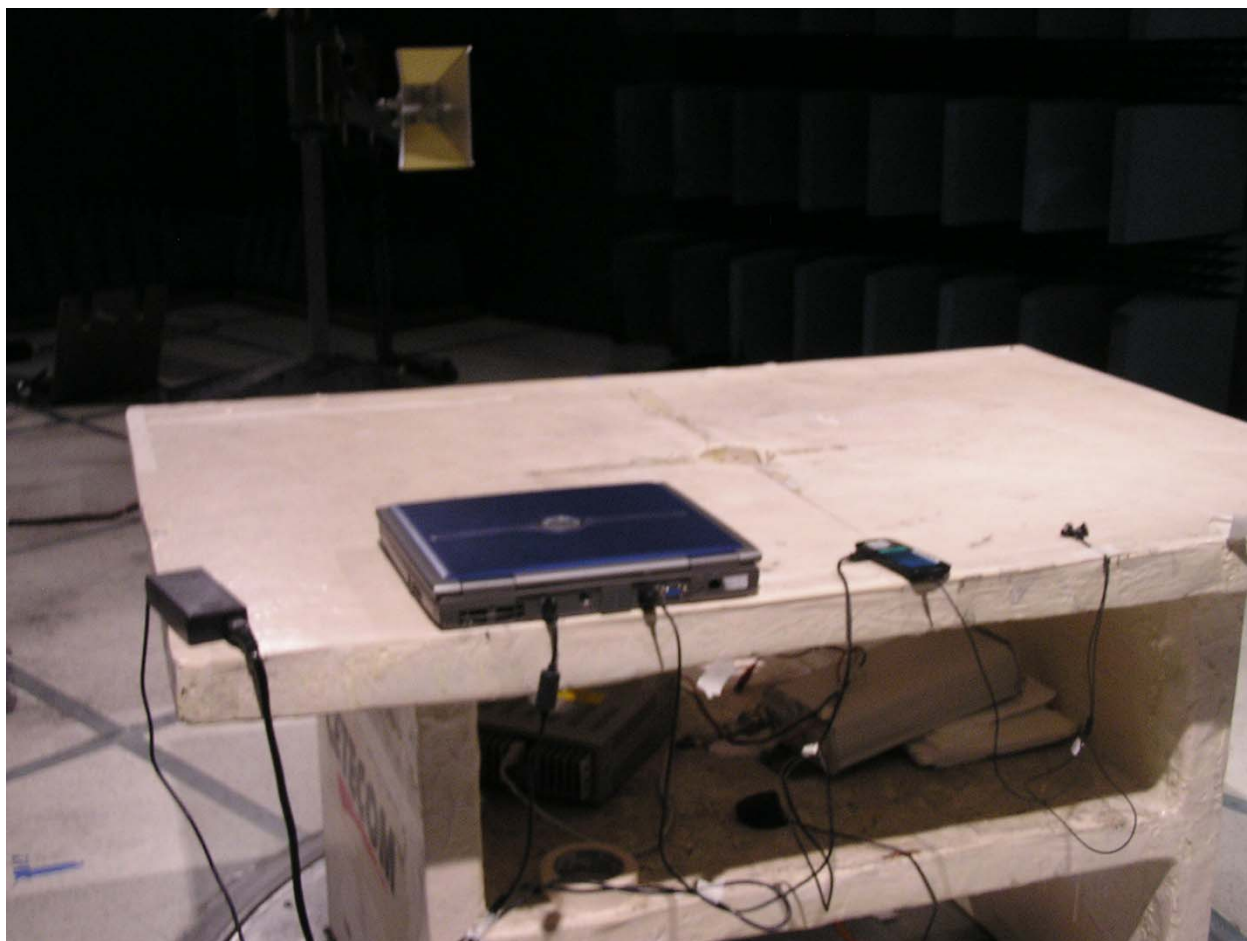
Receiver Radiated Spurious Emissions &gt;1GHz: Standard Cover with laptop
