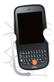
7 Swing the body of the phone out of the back cover as if the right side were a hinge.
