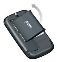
**WARNING** You must remove the battery first whenever you insert or remove the SIM card.
