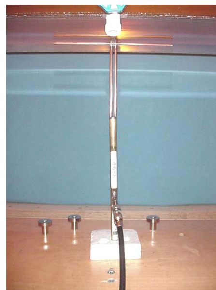
450 MHz Dipole Setup
