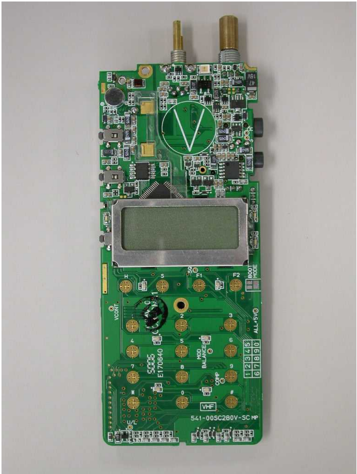
9) MAIN PCB of SC-281 A (Component Side View)
