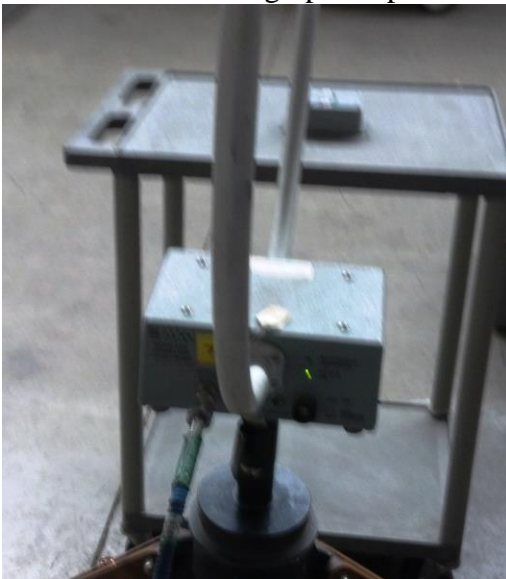
Photograph 2 Spurious Emissions testing using loop antenna
