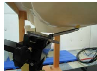
Fig. 17. Head SAR Test Setup
