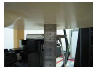
Fig. 21. Body SAR Test Setup with Holster
