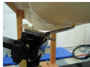
Fig. 18. Head SAR Test Setup
