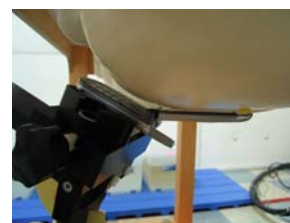
Fig. 16. Head SAR Test Setup
