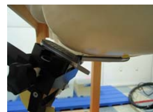
Fig. 15. Head SAR Test Setup
