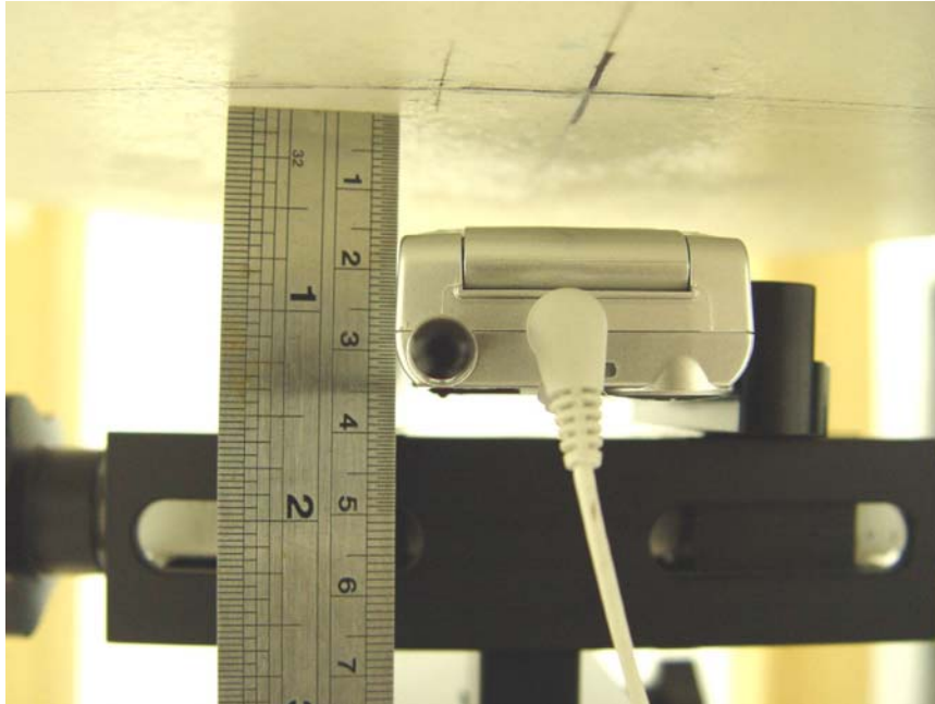
Fig. 9.7 Body Worn-keypad up with 1.5 cm gap
