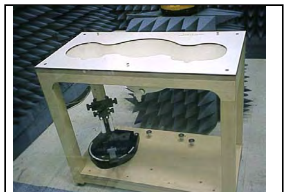
Figure 6. SAM Twin Phantom
