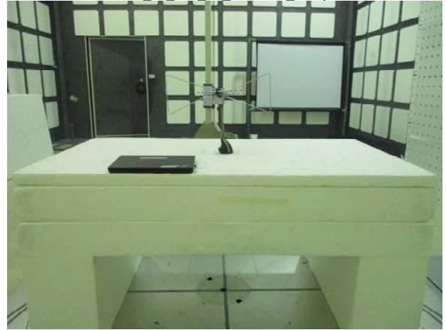
Part 15 247 LE Radiated Setup
