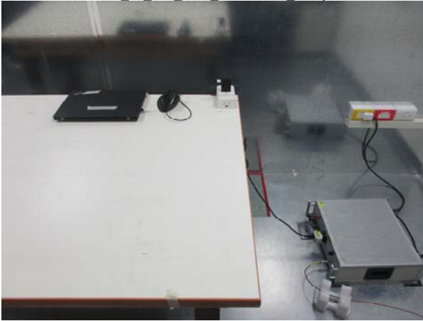
Part 15 249 SRD Conduction Setup
