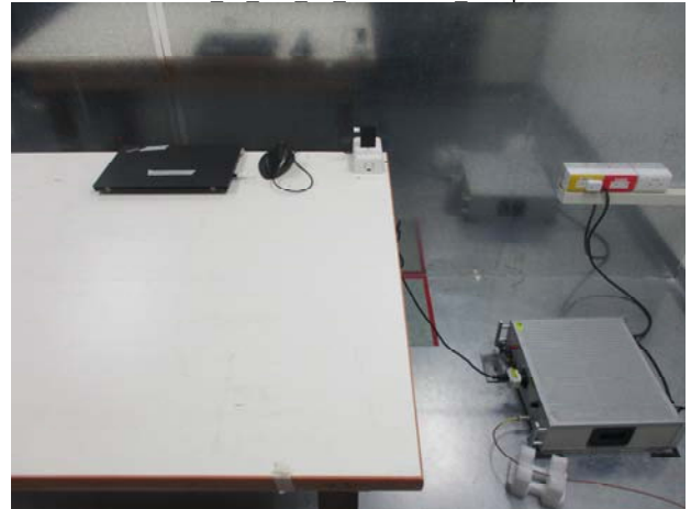
Part 15 247 LE Conduction Setup
