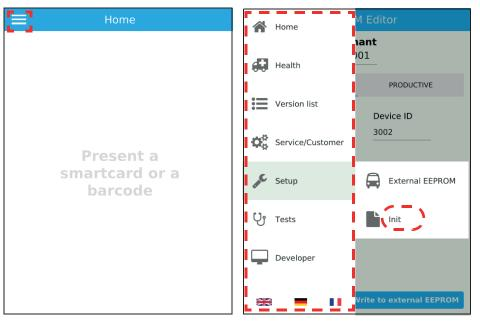
Figure 4-3 BAT - Menu, <Setup>/<Init>
