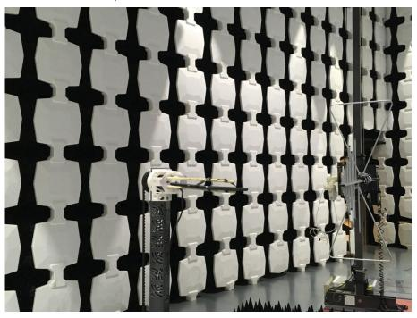
Description: Substitution Antenna for ERP Test
