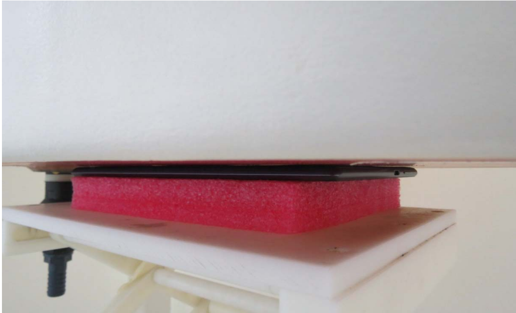
Picture 8: Back Side, the distance from handset to the bottom of the Phantom is 0mm
