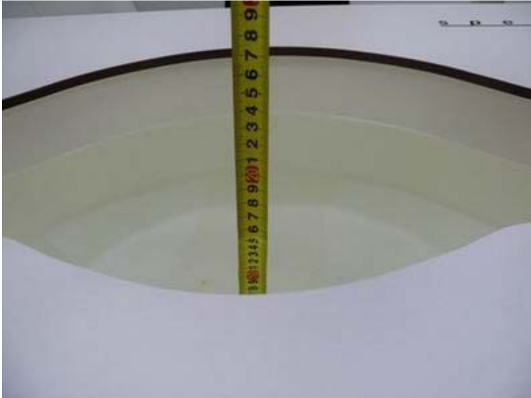
Picture 5: Liquid depth in the flat Phantom (5600 MHz, 15.3cm depth)
