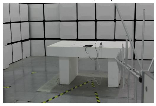
$\textbf{1.3} \ \ \text{Setup for Unwanted Emissions that fall Outside of the Restricted Bands} \\ \text{(Radiated) and Unwanted Emissions in the Restricted Bands} \\ \text{(Radiated) above 1GHz} \\$
