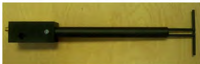
Figure 1 – MVG COMOSAR Validation Dipole
