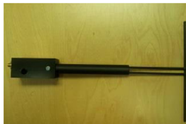
Figure 1 – MVG COMOSAR Validation Dipole
