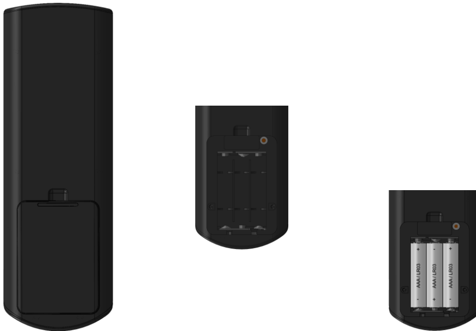
Figure 5: Changing the battery in the RF-TOUCH hand-held remote control
