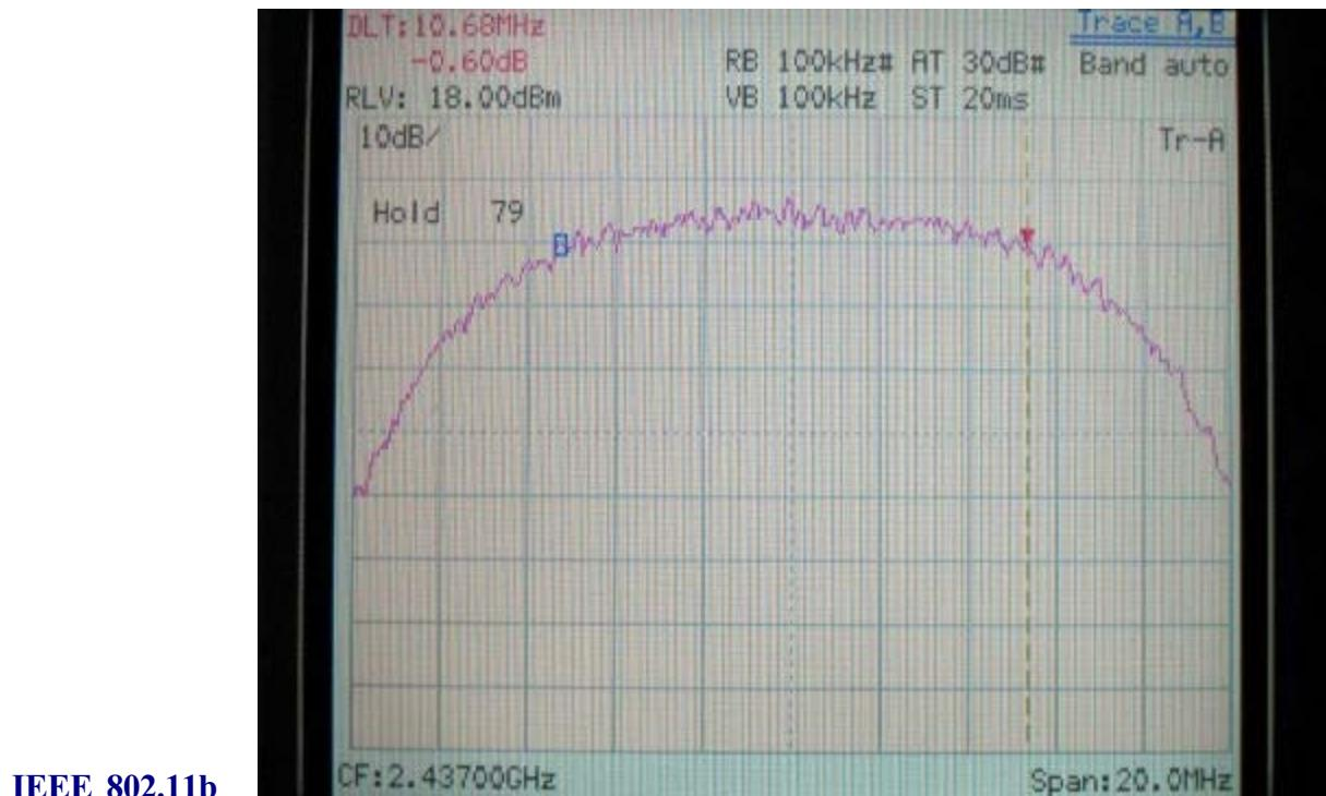
**6dB Bandwidth of Channel 11 (The minimum 6dB BW at least 500kHz)**
