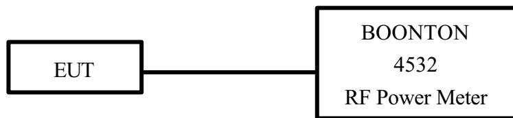
1. The output of the transmitter is connected to the BOONTON RF Power Meter.
