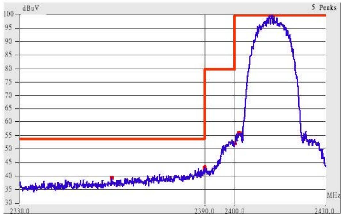
This is the hard copy of our bandedge measurement generated by our bandedge testing program. The plot shown above is the bandedge of channel 1.
