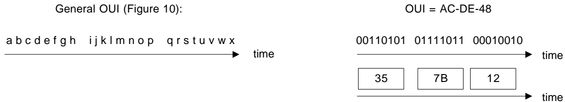
Figure 14—IEEE 802.5 ® , etc., frame: Order of bit and octet transmission for an OUI in a MAC address contained in a MAC Information field (noncanonical format)
