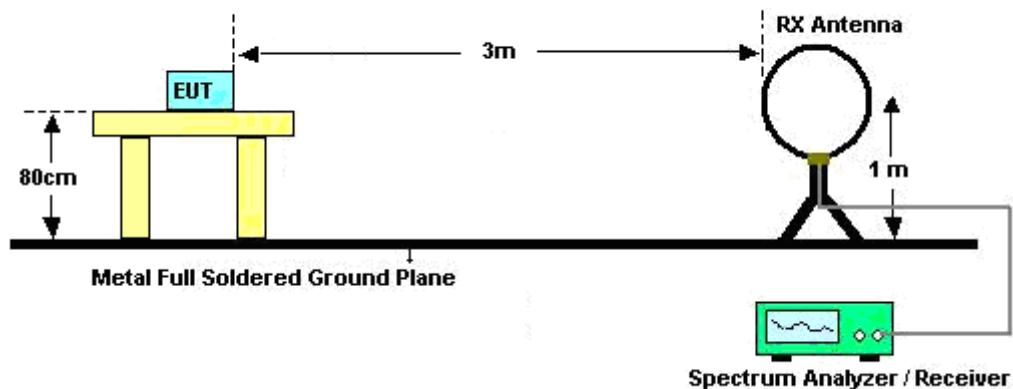
For radiated emissions from 30MHz to 1GHz
