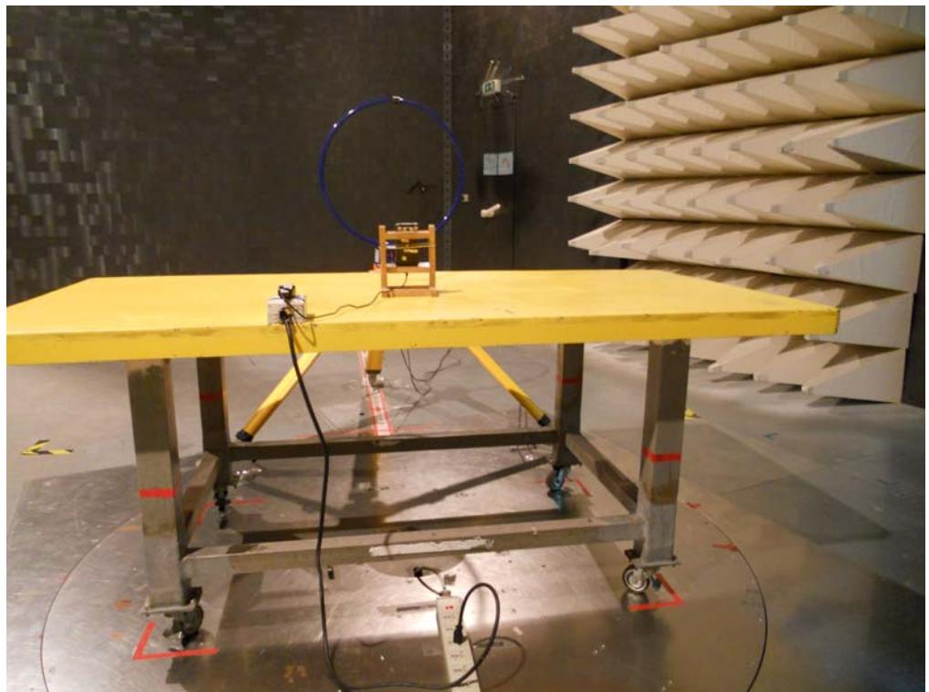
For radiated emissions 9kHz~30MHz
