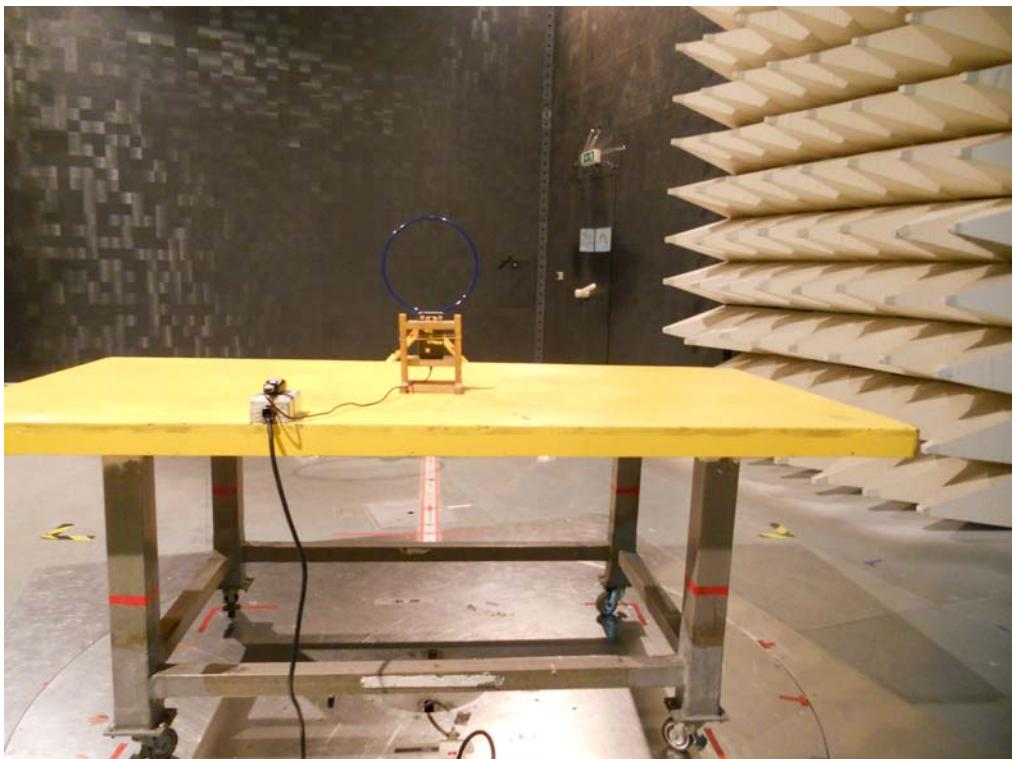
For radiated emissions 30MHz~1GHz
