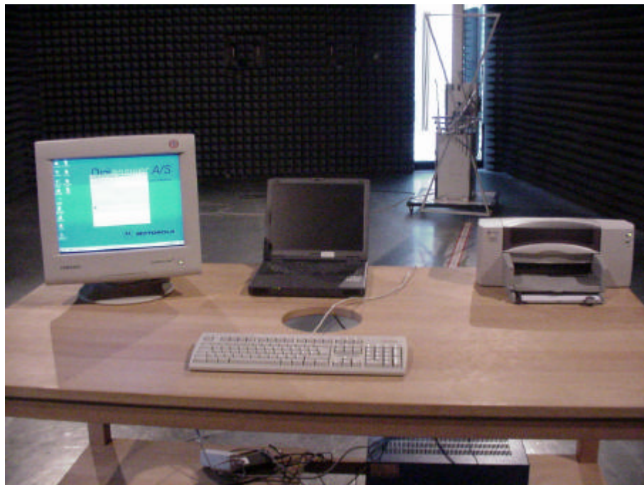
Picture 1 : Setup for radiated emission tests
