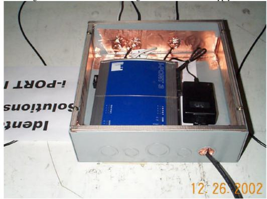
Interior view of NEMA Enclosure, showing the access door of the i-Port III in an "Open" state. Note the bond straps connecting both the door and the RF Bulk Lead of the i-Port III to the i-Port III Chassis. Also, note the RF gasketing on the door edges and on the chassis edges.
