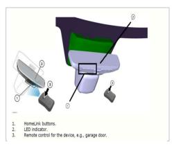
Programming procedure: press the button to be programmed (outlined in 1, 1st, 2nd, or 3rd button) and then release it.
