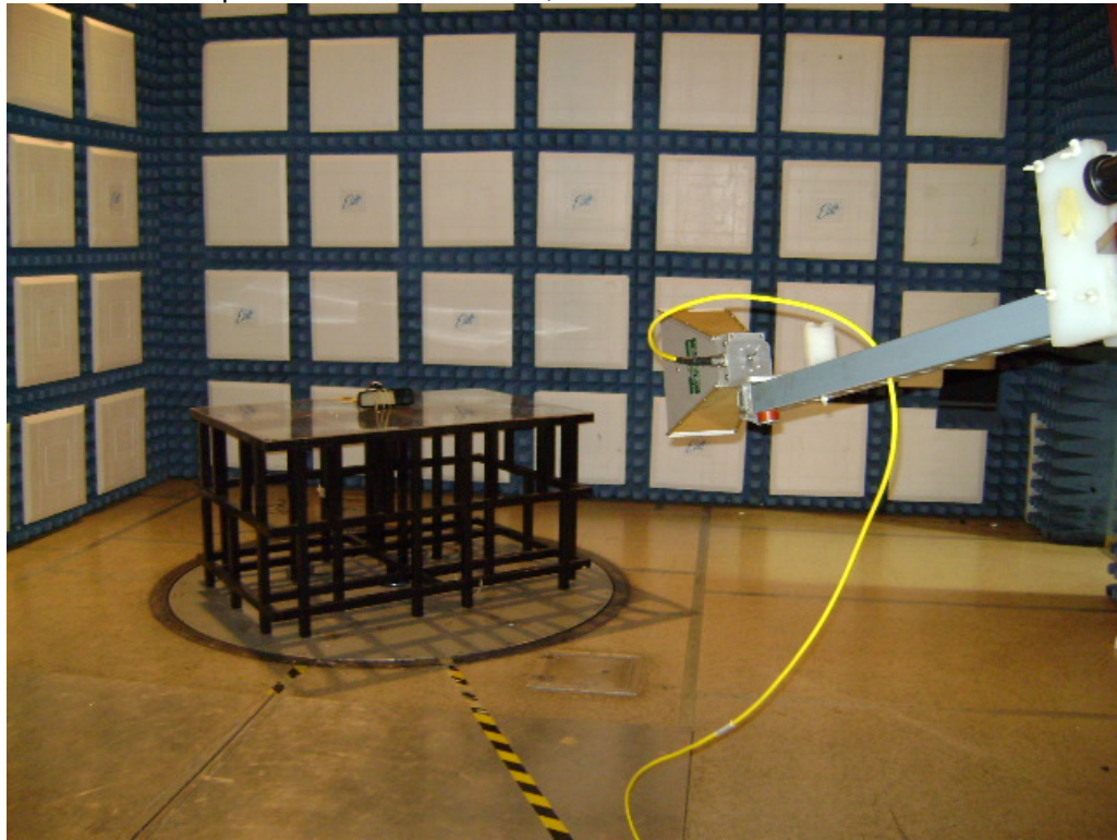
Test Set-up for Radiated Emissions, 1GHz to 5GHz – Horizontal Polarization
