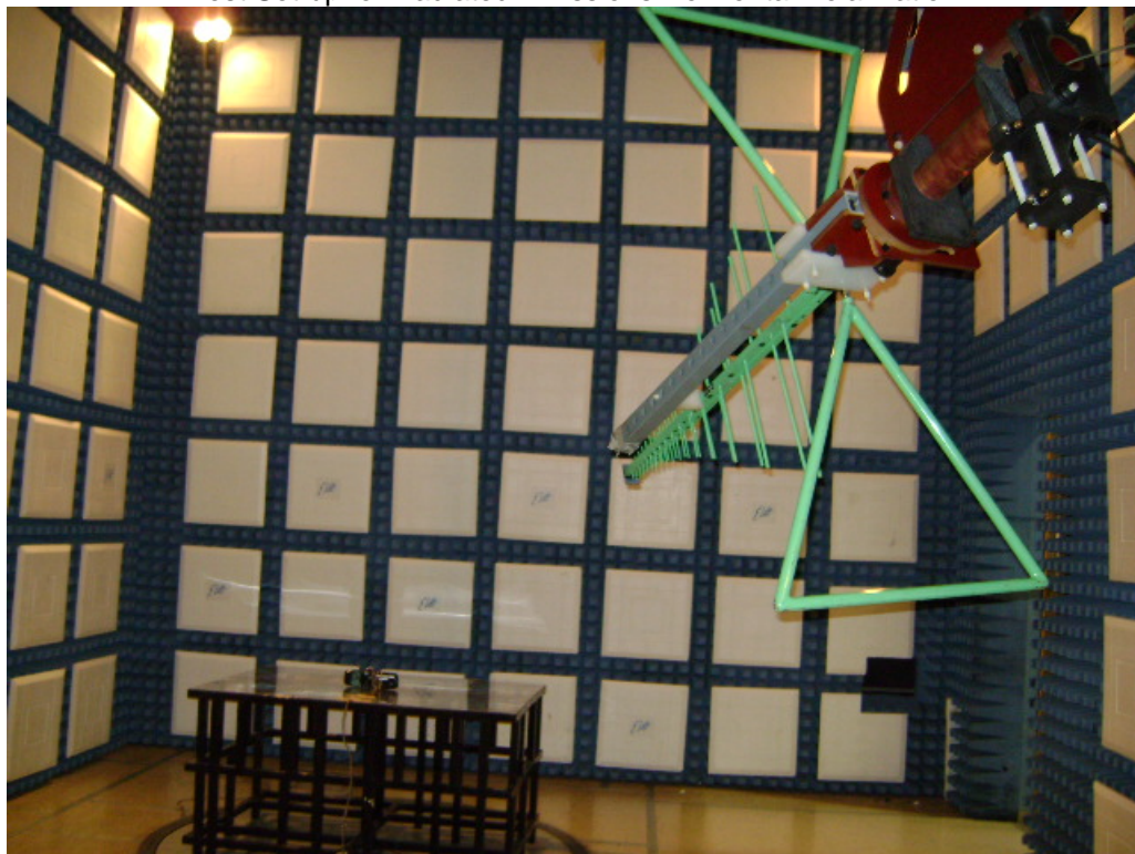
Test Set-up for Radiated Emissions Vertical Polarization
