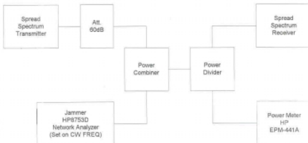
Figure 1. Processing Gain Measurement Setup
