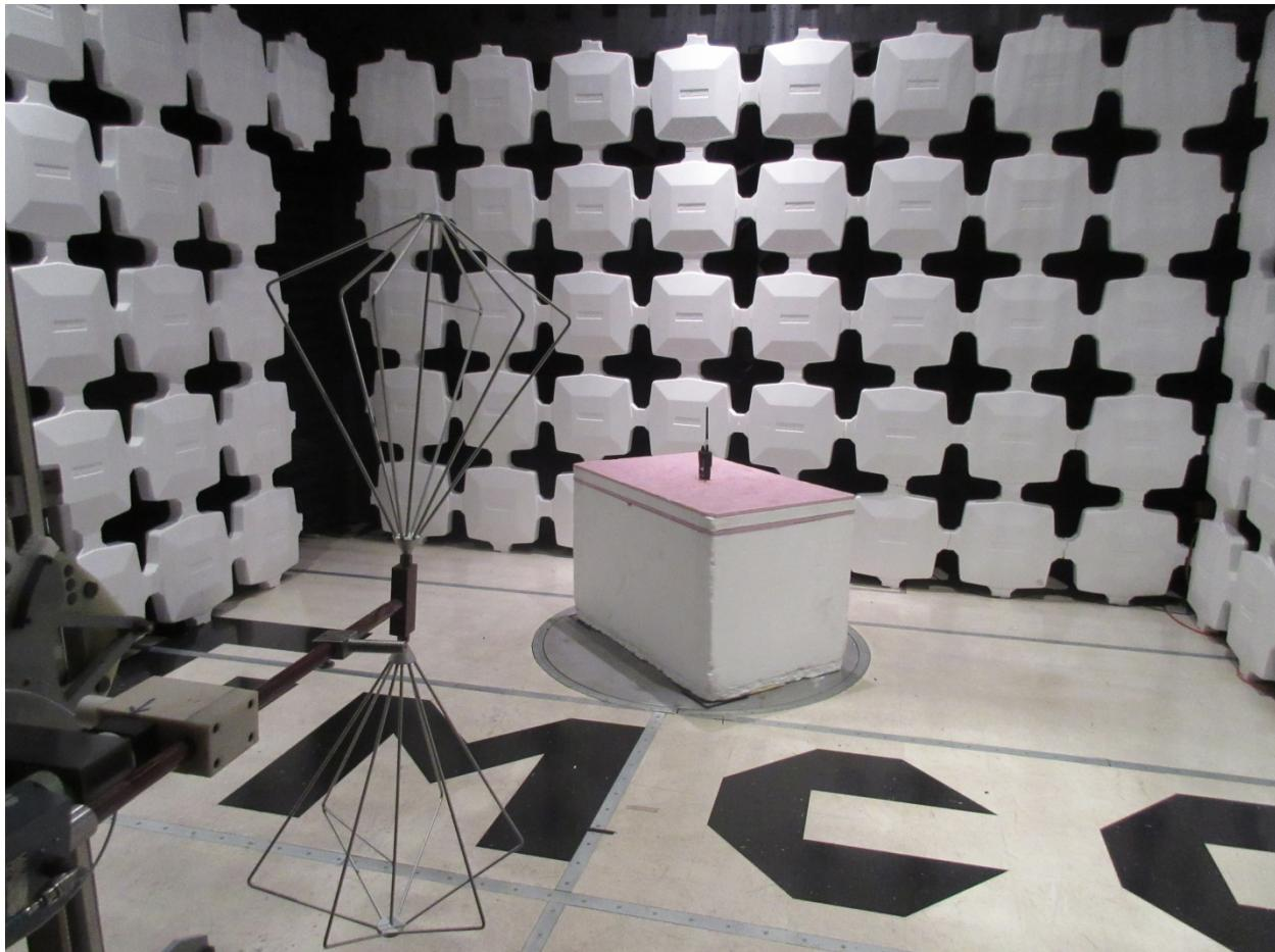
**Radiated Spurious Emissions: 200 MHz – 1 GHz**
