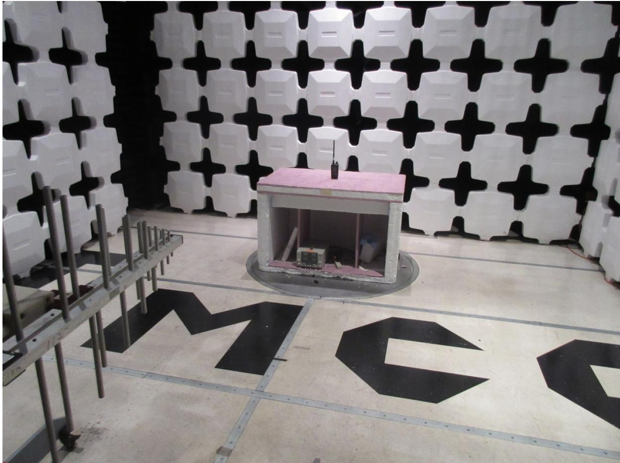
**Radiated Spurious Emissions: 1 GHz – 12.5 GHz**
