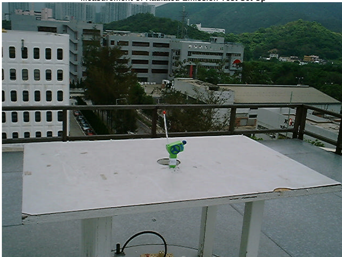
Measurement of Radiated Emission Test Set Up
