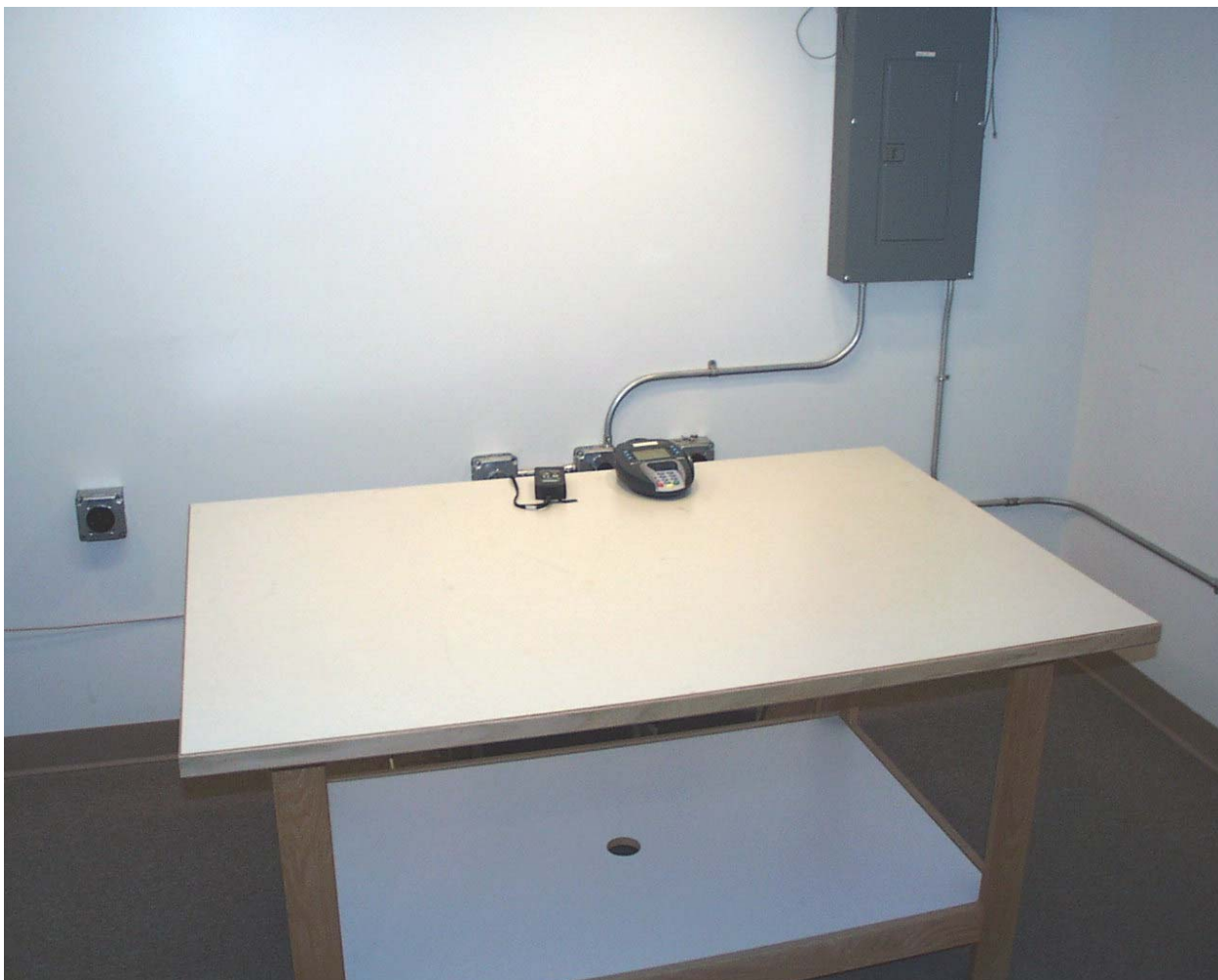
Front View of the Conducted Emission Test Set Up
