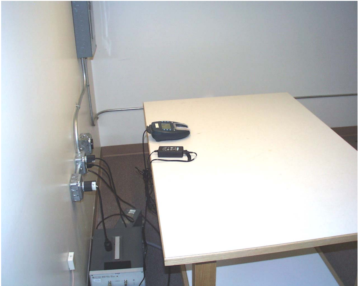
Back View of the Conducted Emission Test Set Up
