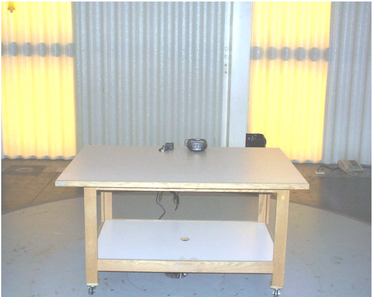
Front View of the Radiated Test Setup (Horizontal Alignment)
