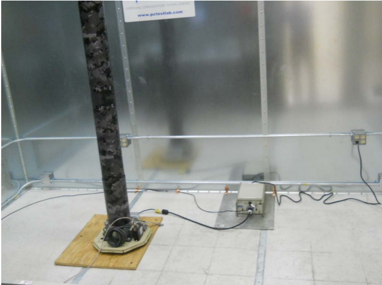
Figure 1. AC Line Conducted Test Setup
