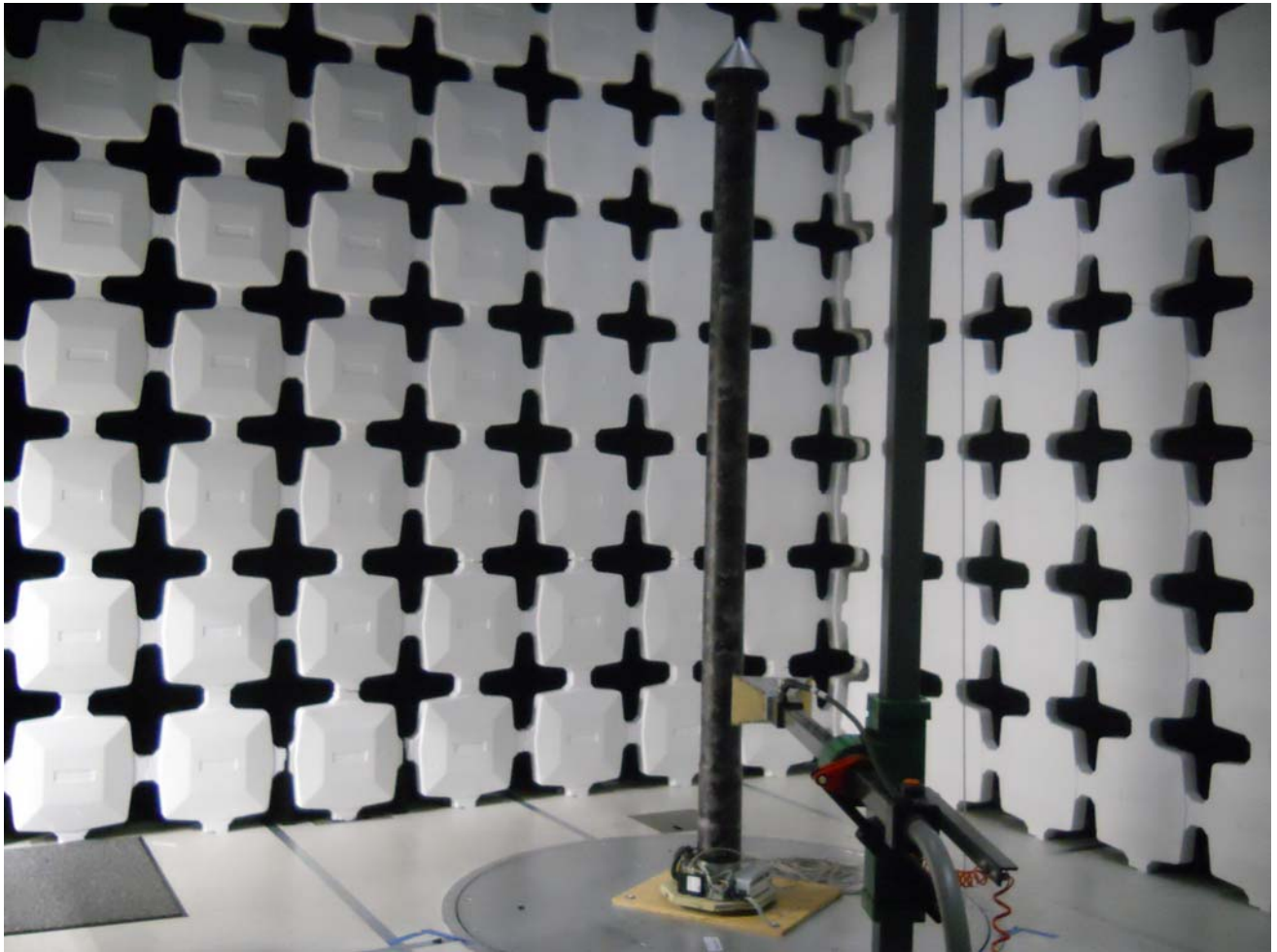
Figure 3. Radiated Emissions Test Setup Above 960MHz (1 meter)
