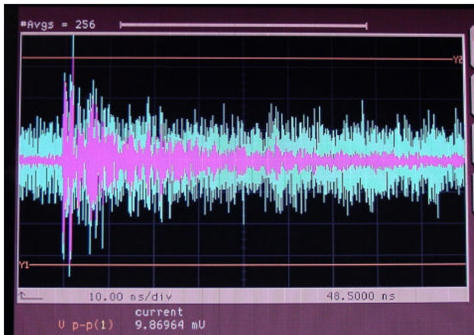
Fig. 5.1: Superimposed traces comparing 4 averaged samples vs. 256 samples per trace
