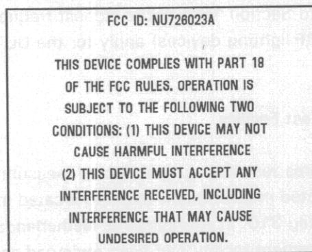
Due to the dimensions of the device, only the FCC identifier is affixed to each item that is marketed for sale. The underneath photograph shows the location of the FCC ID on the lamp. Each production lamp will be permanently marked with the FCC ID. The marks will be applied to the lower plastic housing which is made from white, glass filled PBT plastic. The ink used will be Markem series 5461 ink, colour reference Markem Brilliant Green.
