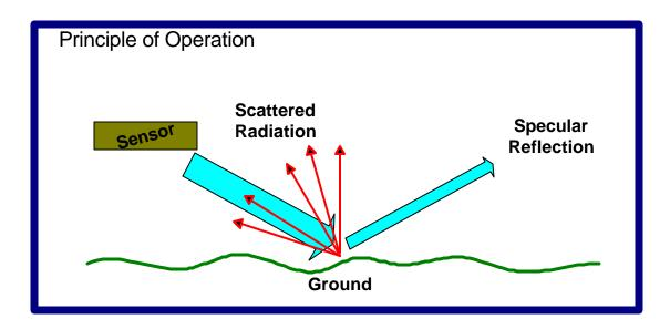
Doppler effect speed sensors are ideal for stubble fields, plowed fields, and gravel roads which give a large amount of scattered radiation, but are less reliable on smooth surfaces such as on concrete or blacktop roads which have a larger amount of specular reflection. This is particularly true if the smooth surface is wet. Doppler effect speed sensors do not work if the incident surface is standing water.
