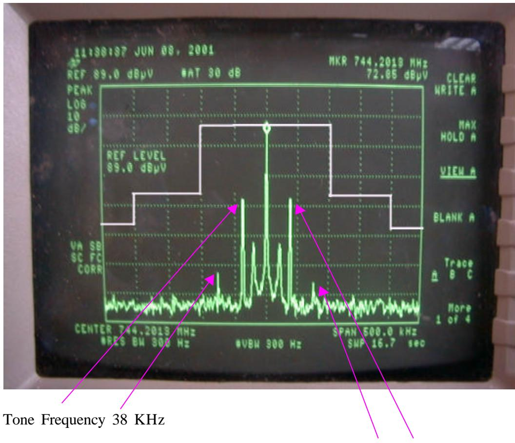
Firstly, the page 31 of report is actually for 15 KHz. Because, the EUT is including tone frequency 38kHz when unmodulation then input 15 kHz signal by signal generator..
