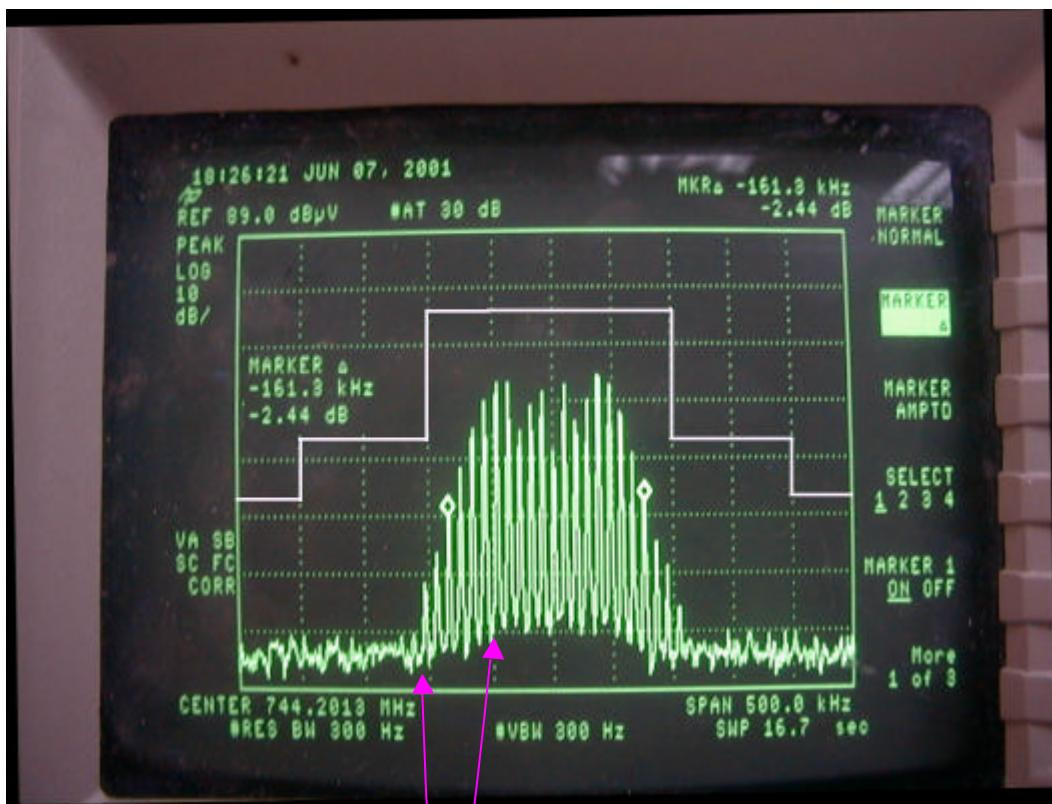
The sidebands spaced is including the 15kHz and all harmonic frequency with 38 kHz tone frequency
