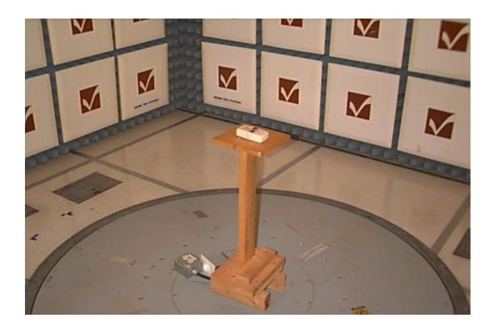
view of the Remote Control transmitter during the Radiated Emissions tests. This view shows the orientation of the product where the maximum signal levels were present (horizontal polarity).
