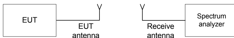
Figure 7.4.1 Band edge emission test setup
