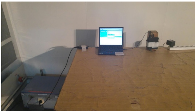
Photograph 8.1.1 Setup for conducted emission measurements
