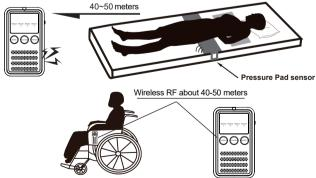
b. Pre-warning testing (For 636): The simulated human body lies on the pressure pad sideways or moves to the warning area at both ends of the pressure pad placed on the edge of the bed. In that case, the pressure pad sensor detects that the human body will falling from the bed is in danger and immediately sends a signal to activate the alarm main unit to prompt family members or caregivers to adjust the bed position of the caregivered to the safe area in the center of the bed.
