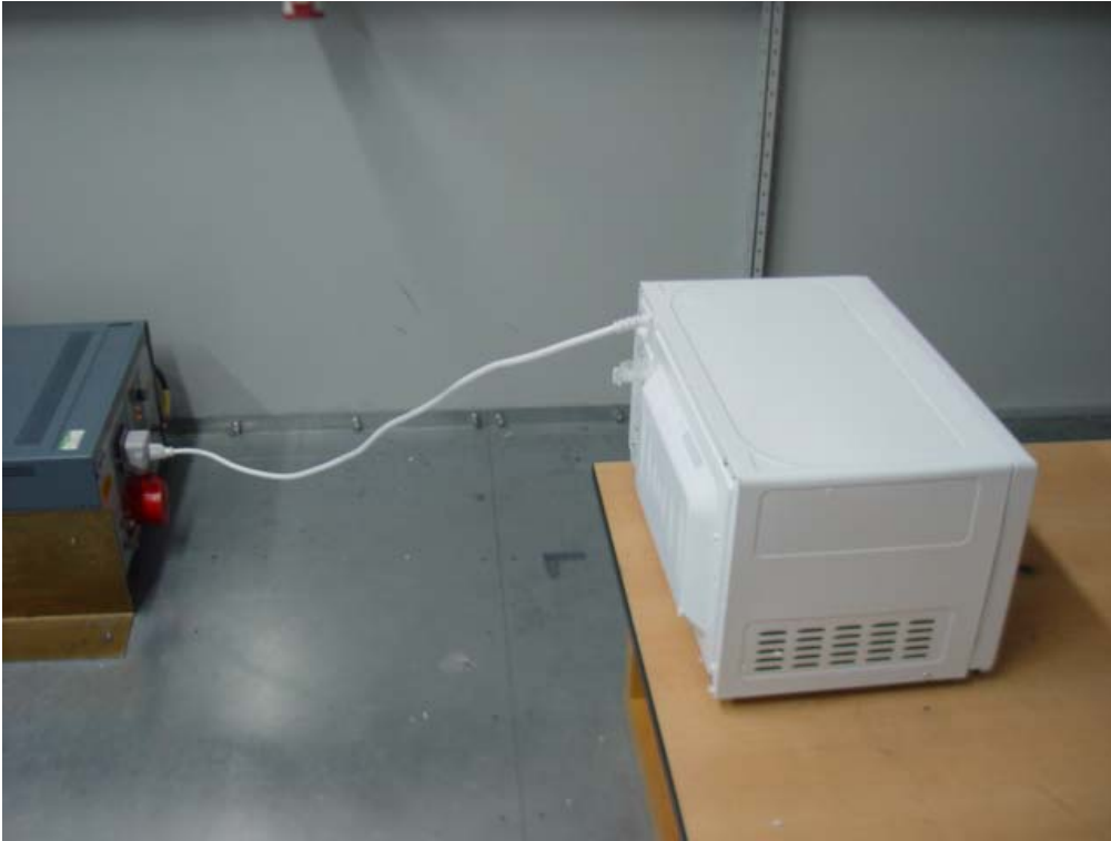
Photo 4 Conducted Disturbance Test (WP700D-S20)
