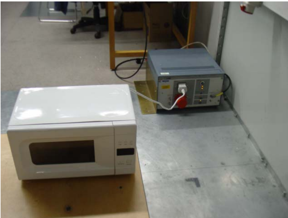
Photo 4 Conducted Disturbance Test (WP700D-S20)
