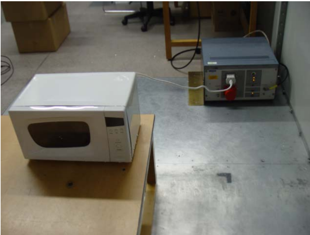
Photo 2 Conducted Disturbance Test (WP700D-N20)
