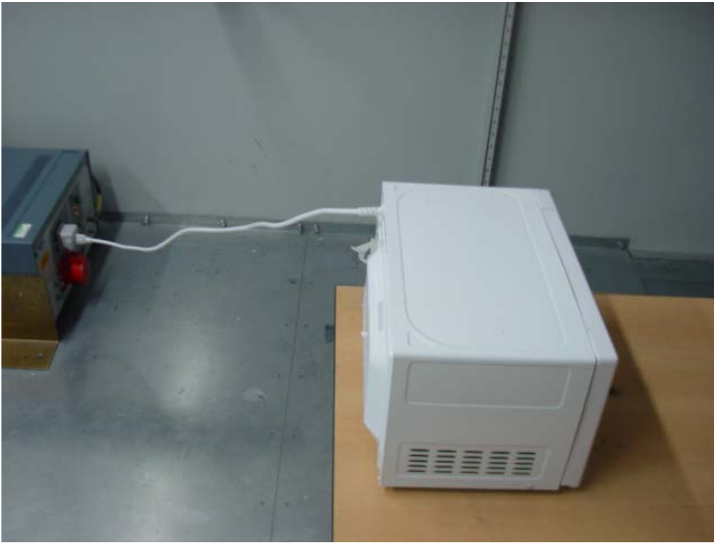
Photo 2 Conducted Disturbance Test (WP700D-N20)
