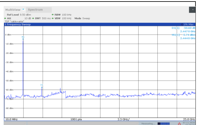
Conducted spurious emissions 10MHz – 25GHz , ch2441MHz, 4_PI_8DPSK
