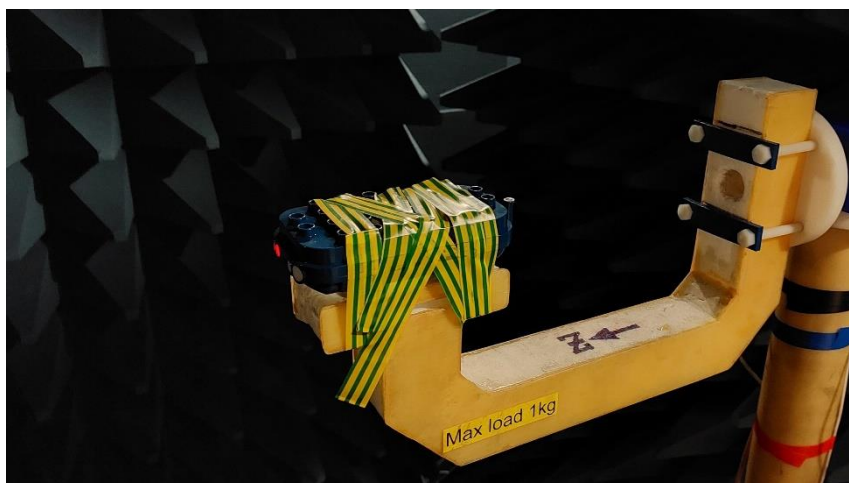
Figure 4: Placement of AUT on turn arm in chamber (additional view)
