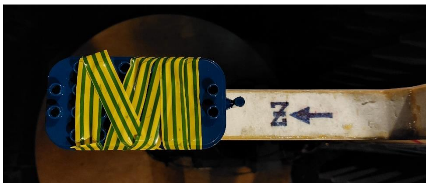
Figure 3: Placement of AUT on turn arm in chamber showing Z-axis
