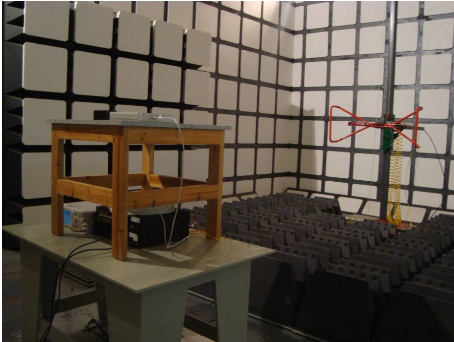
Below 1 GHz: Spurious Radiated Emissions – Rear View
