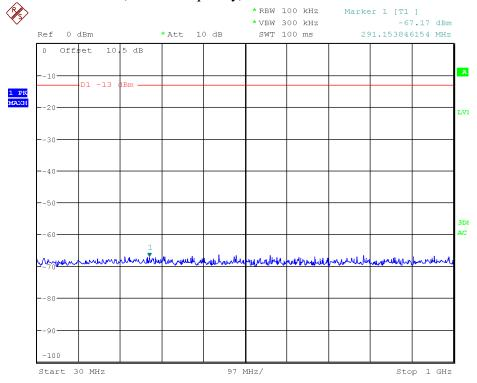
2100MHz -LTE-5M downlink (middle frequency) Above 1GHz
