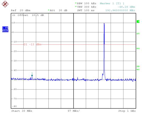
700MHz -LTE-5M downlink (highest frequency) Above 1GHz
