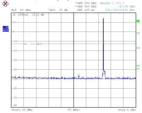
700MHz -LTE-1.4M downlink (lowest frequency) Above 1GHz
