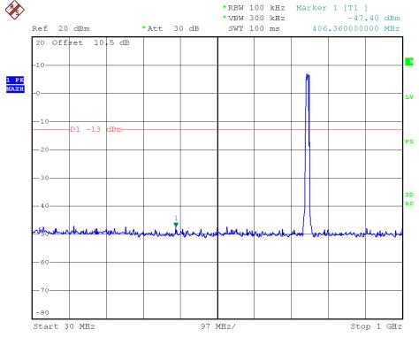
700MHz –LTE-10M downlink (lowest frequency) Above 1GHz
