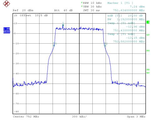
700MHz-LTE –1.4M downlink (highest frequency )-Input
