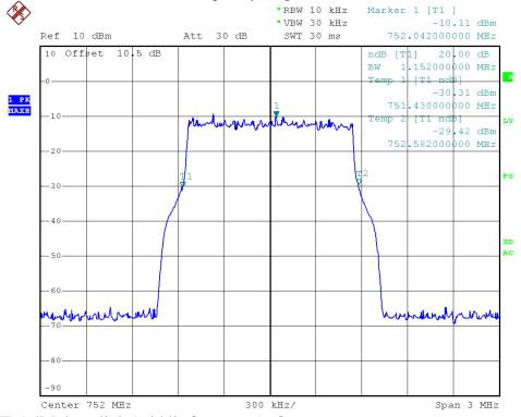
700MHz-LTE-1.4M downlink (middle frequency)- Output
