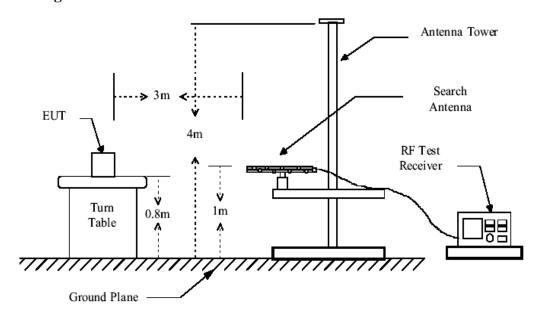
Figure 1. 30 MHz to 1GHz radiated emissions test configuration
