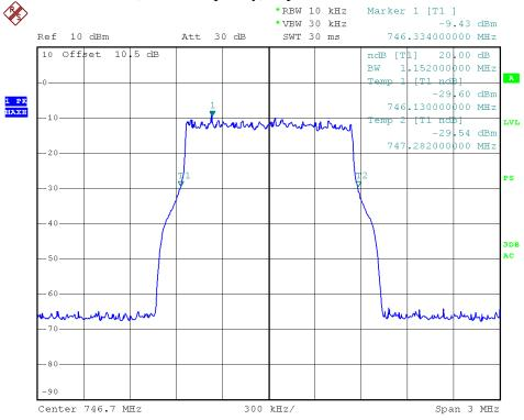
700MHz-LTE-1.4M downlink (lowest frequency)-Output
