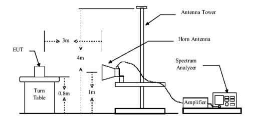
Figure 2. Above 1GHz radiated emissions test configuration
