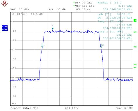
700MHz-LTE-3M downlink (highest frequency)- Output
