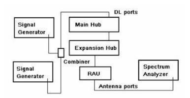
Fig.1 Down Link Intermodulation
