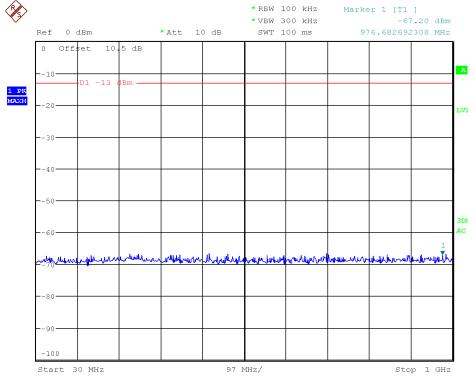
2100MHz -LTE-1.4M downlink (highest frequency) Above 1GHz
