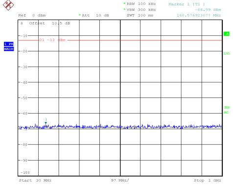
2100MHz –LTE-3M downlink (highest frequency) Above 1GHz
