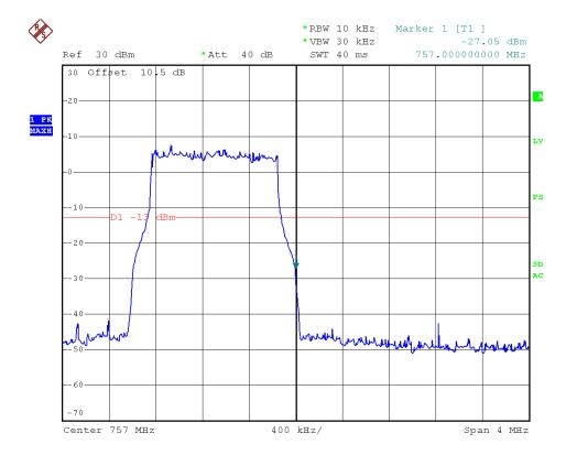
700MHz-LTE-3M Channel Bandwidth -Lower Edge
