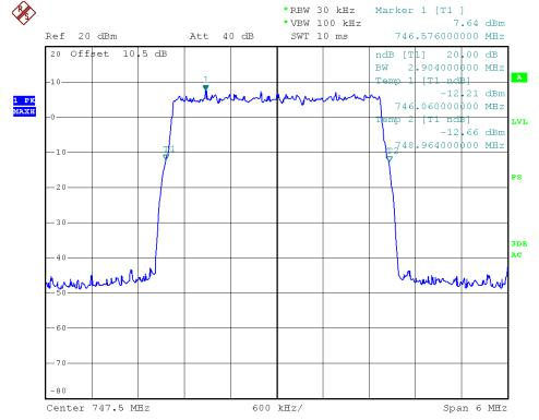
700MHz-LTE-3M downlink (middle frequency)-Input
