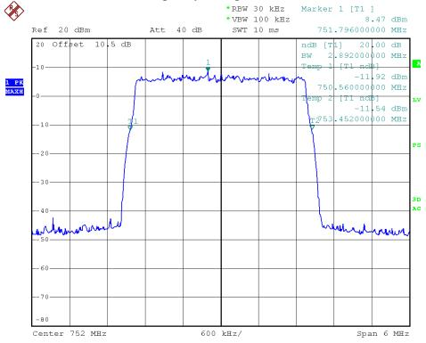
700MHz-LTE-3M downlink (highest frequency)-Input
