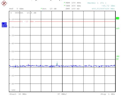
2100MHz –LTE-5M downlink (highest frequency) Above 1GHz
