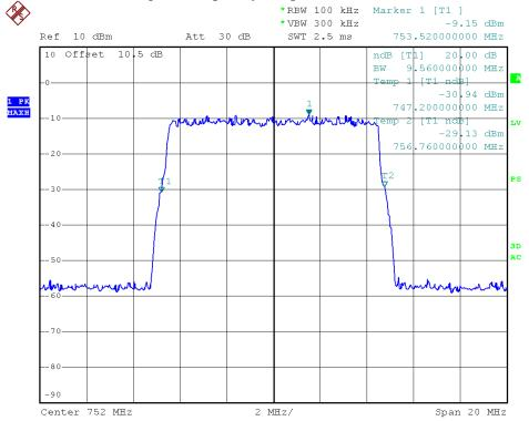
700MHz-LTE-10M downlink (highest frequency)- Output
