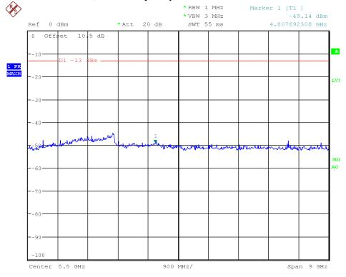
700MHz -LTE-1.4M downlink (highest frequency) 30MHz-1GHz
