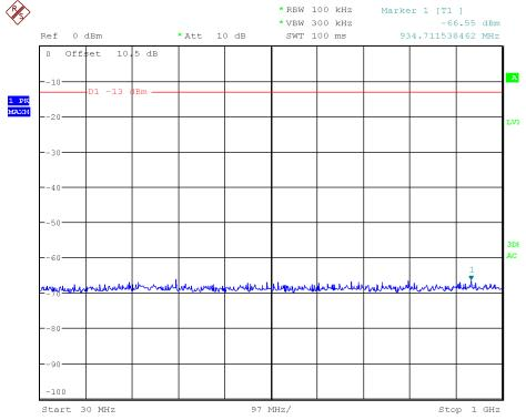
2100MHz -LTE-5M downlink (lowest frequency) Above 1GHz
