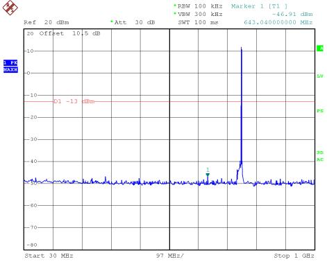
700MHz -LTE-3M downlink (highest frequency) Above 1GHz
