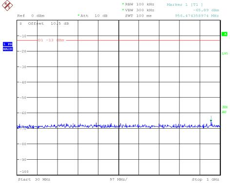
2100MHz -LTE-1.4M downlink (middle frequency) Above 1GHz
