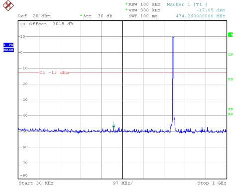
700MHz -LTE-5M downlink (middle frequency) Above 1GHz
