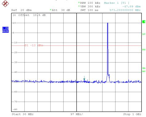
700MHz -LTE-3M downlink (lowest frequency) Above 1GHz
