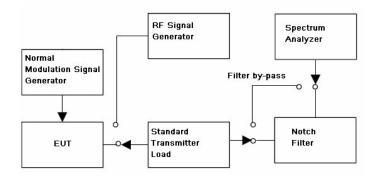
Conducted Emission test procedure:
