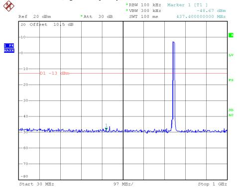
700MHz –LTE-10M downlink (highest frequency) Above 1GHz
