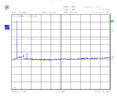
2100MHz –LTE-1.4M downlink (highest frequency) 30MHz-1GHz
