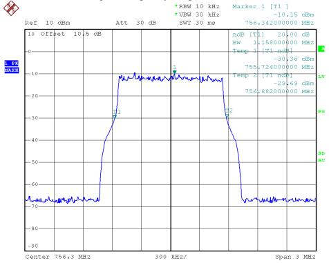
700MHz-LTE-1.4 downlink (highest frequency)- Output
