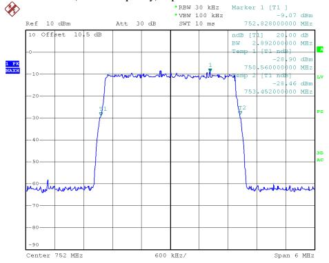
700MHz-LTE-3M downlink (middle frequency)- Output
