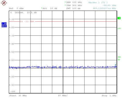
2100MHz -LTE-3M downlink (lowest frequency) Above 1GHz
