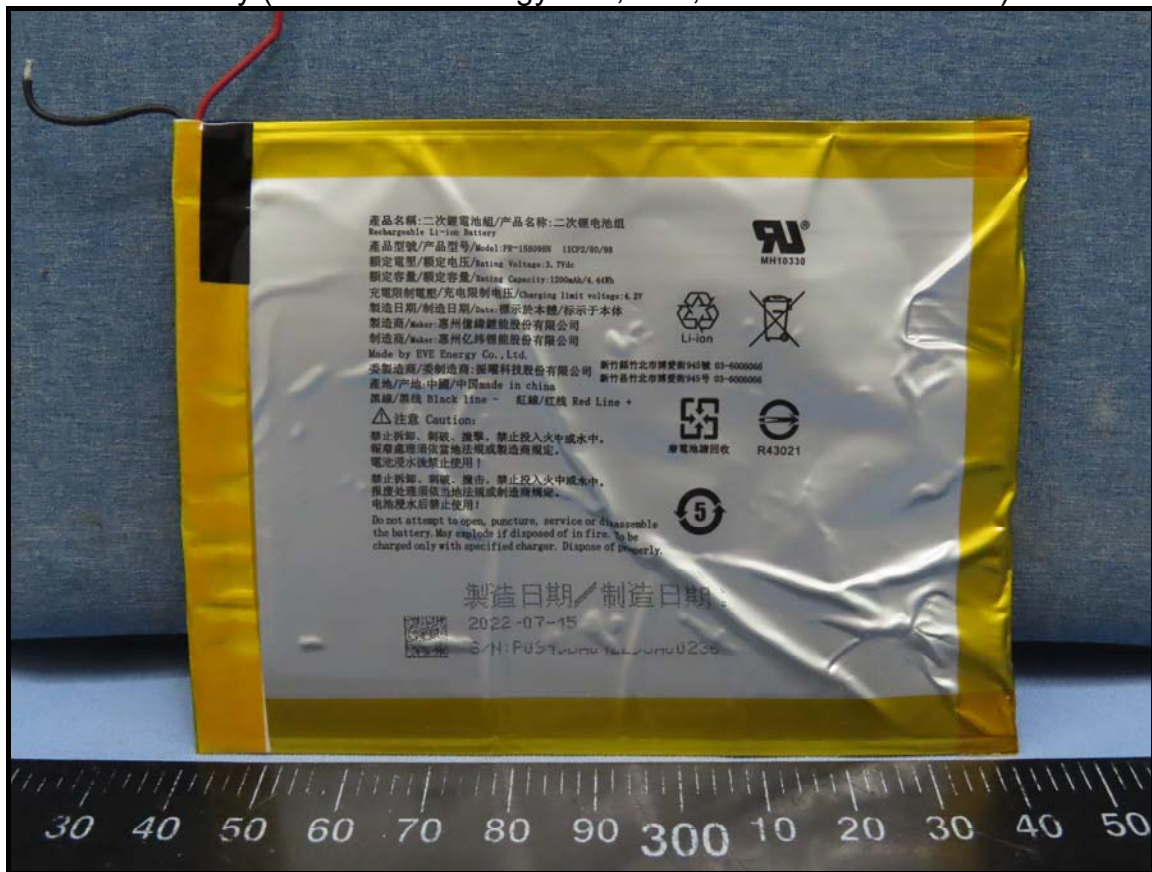
Battery (Brand: EVE Energy CO., LTD, Model: PR-158098N)
