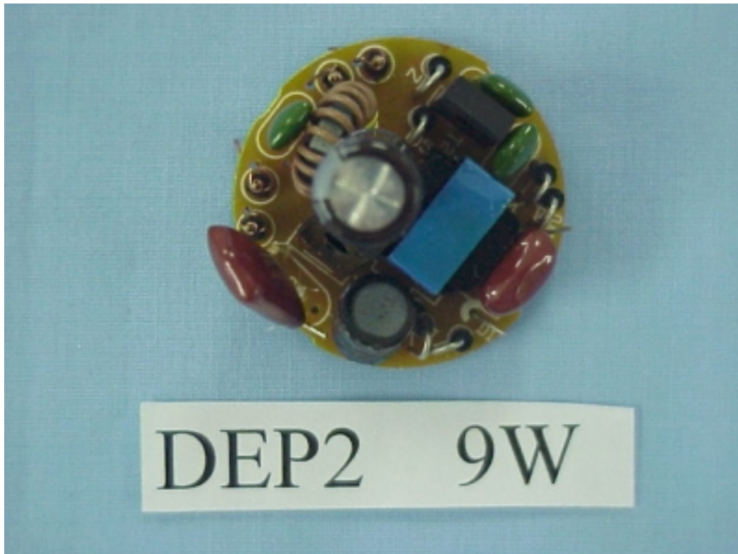
FIGURE 11 ELECTRONIC ENERGY SAVING LAMP (M/N: DEP2/9W) MAIN BOARD (COMPONENT SIDE)
