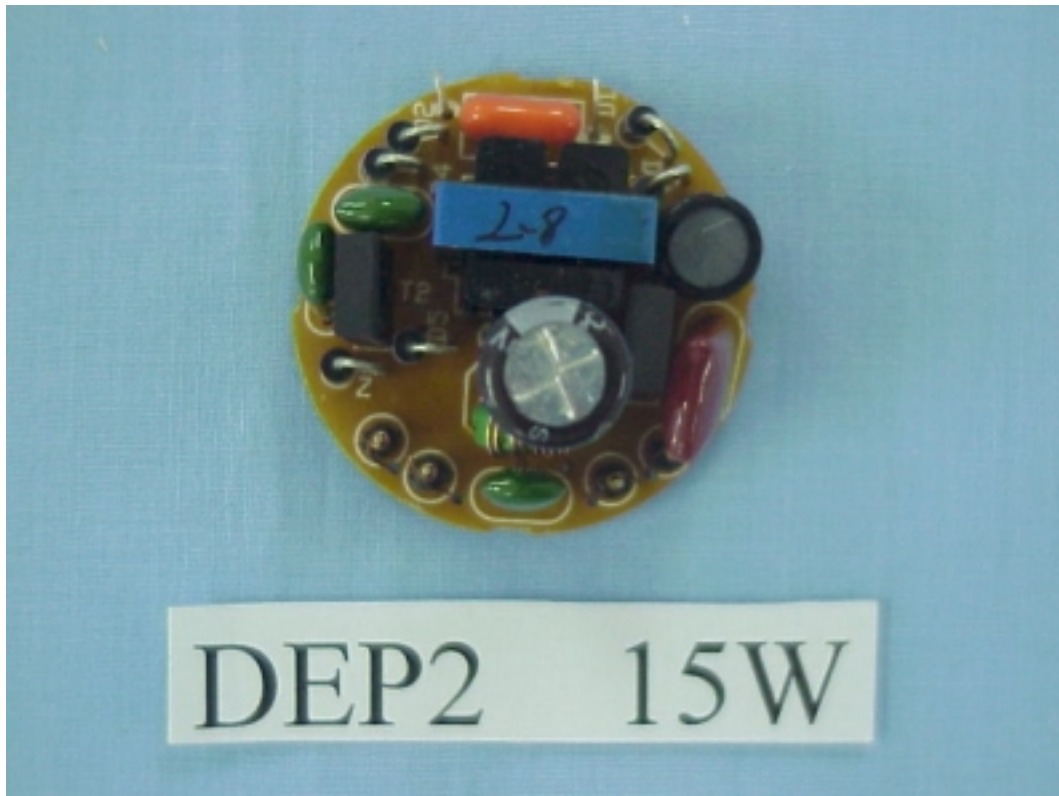
FIGURE 6 ELECTRONIC ENERGY SAVING LAMP (M/N: DEP2/15W) MAIN BOARD (COMPONENT SIDE)
