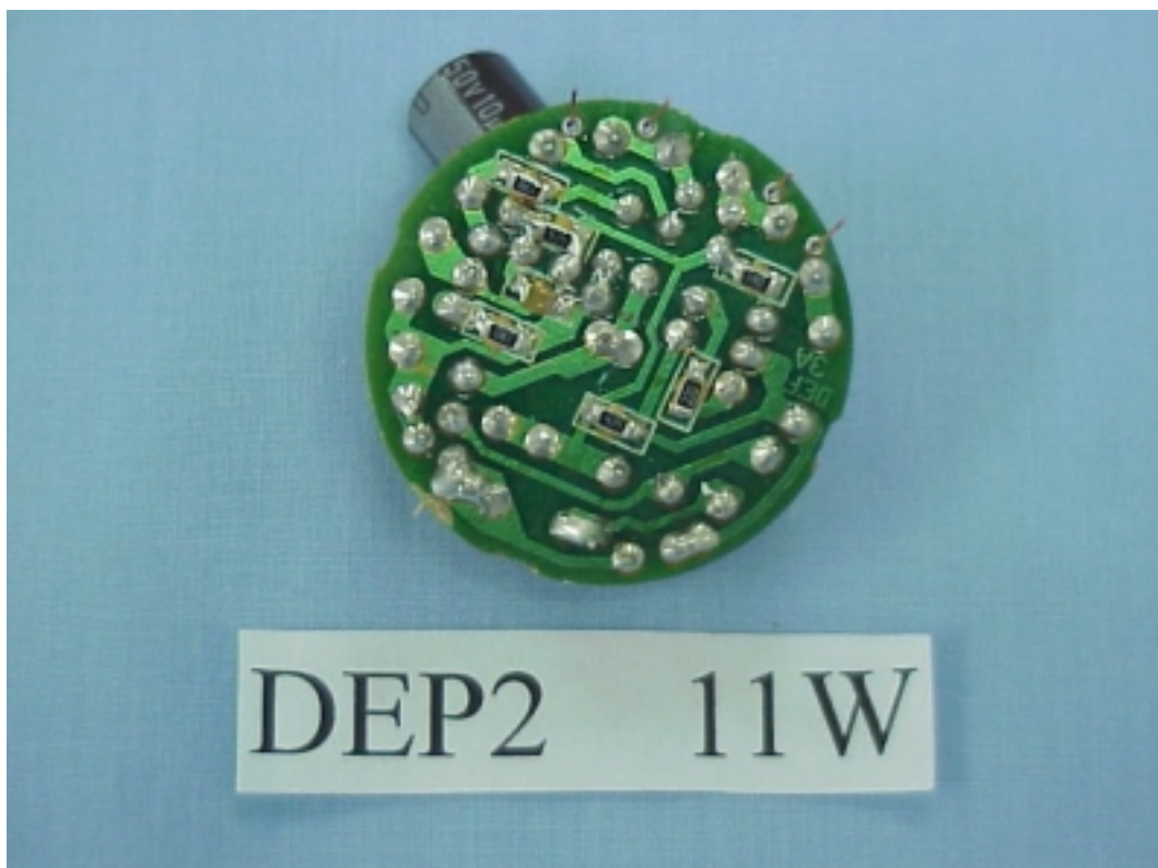
FIGURE 5 ELECTRONIC ENERGY SAVING LAMP (M/N: DEP2/11W) MAIN BOARD (SOLDERED SIDE)
