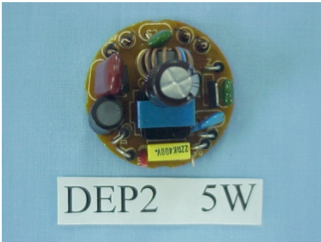
FIGURE 2 ELECTRONIC ENERGY SAVING LAMP (M/N: DEP2/5W) MAIN BOARD (COMPONENT SIDE)
