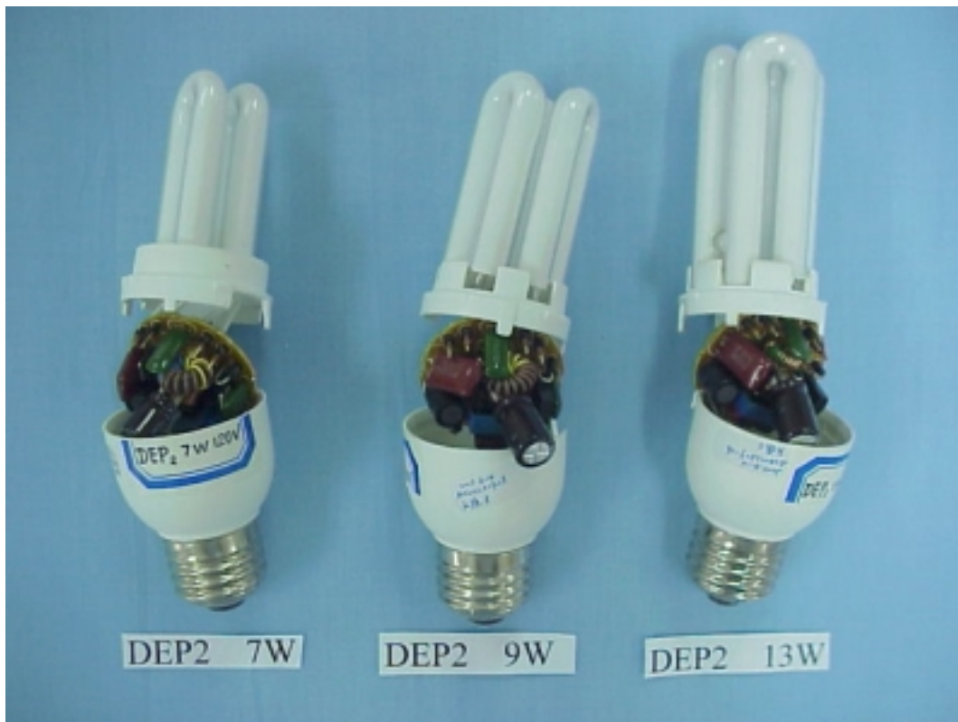
FIGURE 8 ELECTRONIC ENERGY SAVING LAMP (M/N: DEP2/7W, 9W, 13W) COVER REMOVED
