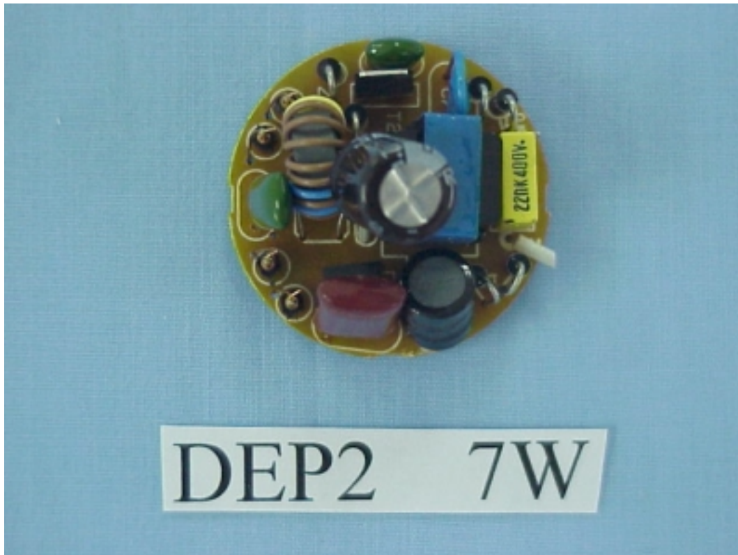
FIGURE 9 ELECTRONIC ENERGY SAVING LAMP (M/N: DEP2/7W) MAIN BOARD (COMPONENT SIDE)
