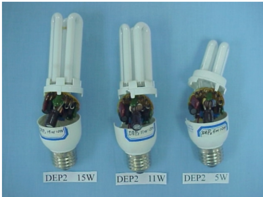
FIGURE 1 ELECTRONIC ENERGY SAVING LAMP (M/N: DEP2/5W, 11W, 15W) COVER REMOVED
