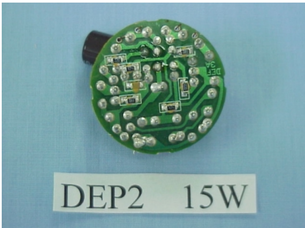
FIGURE 7 ELECTRONIC ENERGY SAVING LAMP (M/N: DEP2/15W) MAIN BOARD (SOLDERED SIDE)
