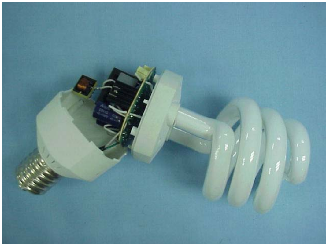
FIGURE 10 ELECTRONIC ENERGY SAVING LAMP (M/N: DEC 3E39 45W) COVER REMOVED
