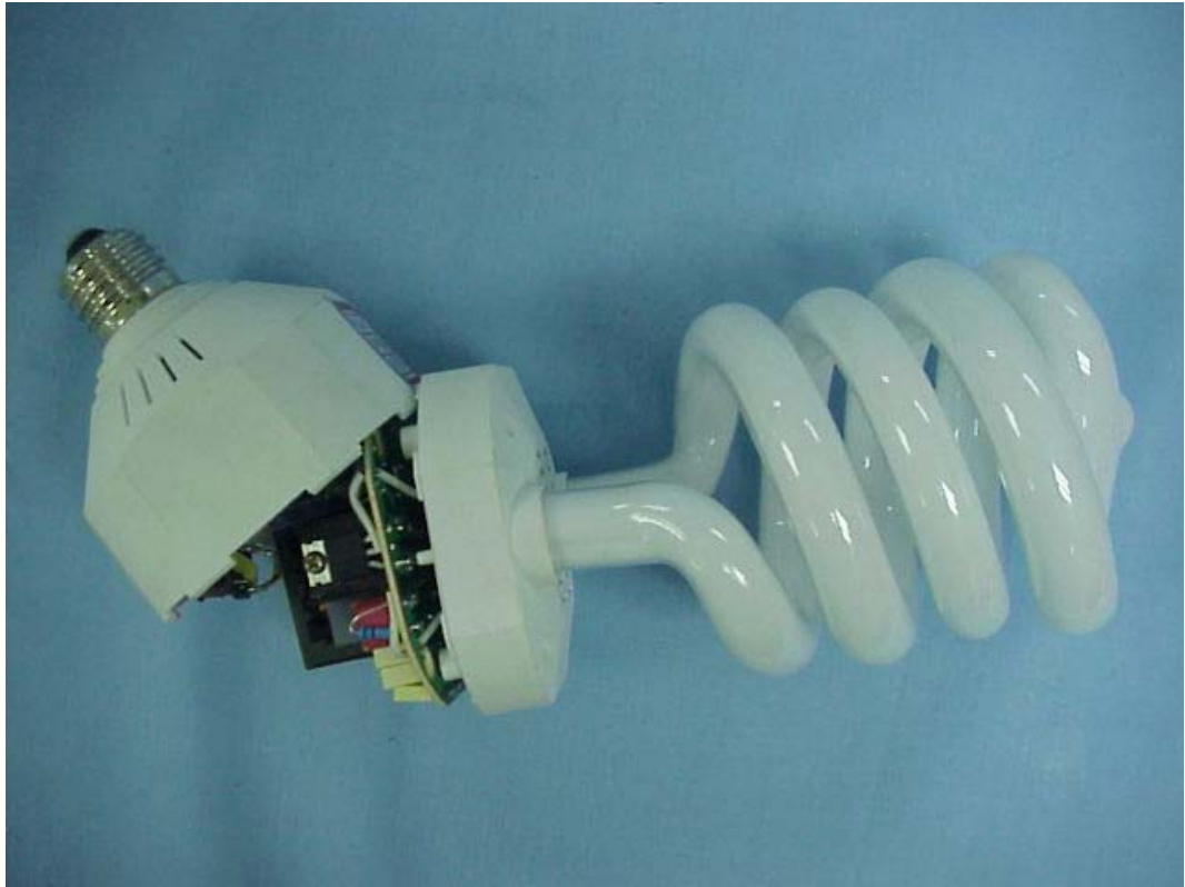
FIGURE 4 ELECTRONIC ENERGY SAVING LAMP (M/N: DEC 3E26 65W) COVER REMOVED
