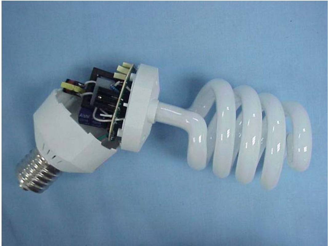
FIGURE 16 ELECTRONIC ENERGY SAVING LAMP (M/N: DEC 3E39 85W) COVER REMOVED
