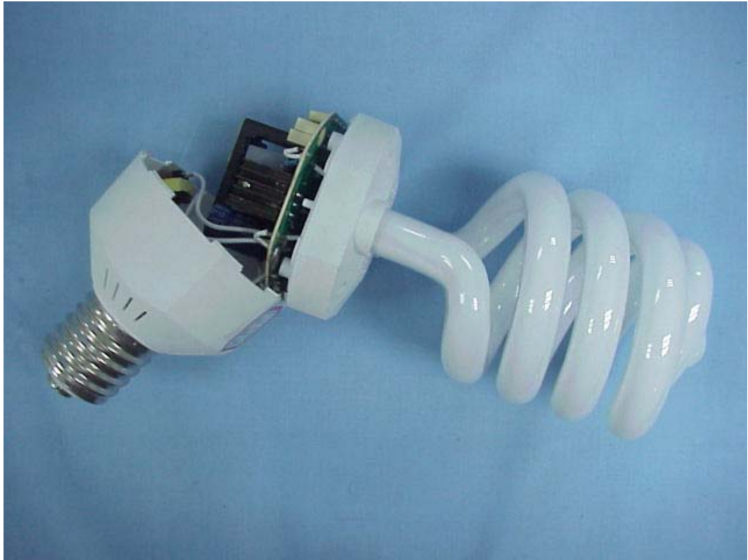
FIGURE 13 ELECTRONIC ENERGY SAVING LAMP (M/N: DEC 3E39 65W) COVER REMOVED
