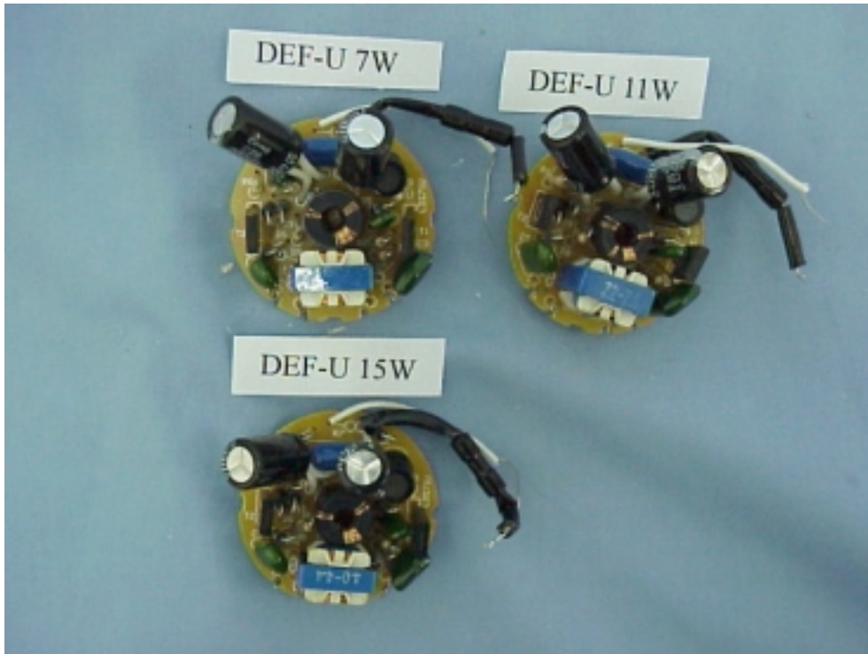
Figure 5 Electronic Energy Saving Lamp (M/N: DEF-U SERIES) MAIN BOARD (COMPONENT SIDE)
