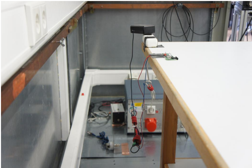
Picture 2: EUT, setup conducted emissions (rear view)
