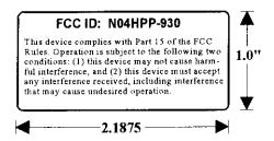
Specifications: Text is black in color and is left justified. Labels are printed in indelible ink on permanent adhesive backing and shall be affixed at a conspicuous location on the EUT.
