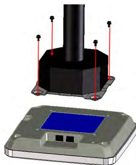
Note: Make sure the arrow on the main bracket is aligned so that it is pointing toward the top side of the Access Point.
