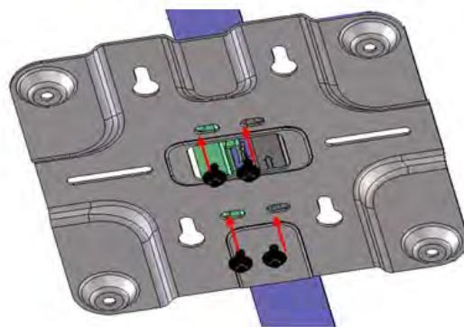
4. Align the screw holes on the main bracket with the corresponding holes on the back of the Access point, then use four M4 screws to attach the main bracket to the Access Point.
