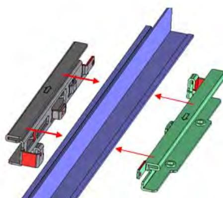
2. After the adapter brackets are affixed onto the T-bar, slide the brackets in the direction of the arrows on the brackets until they are securely attached to each other. Refer to the images below for how the adapter brackets should fit.
