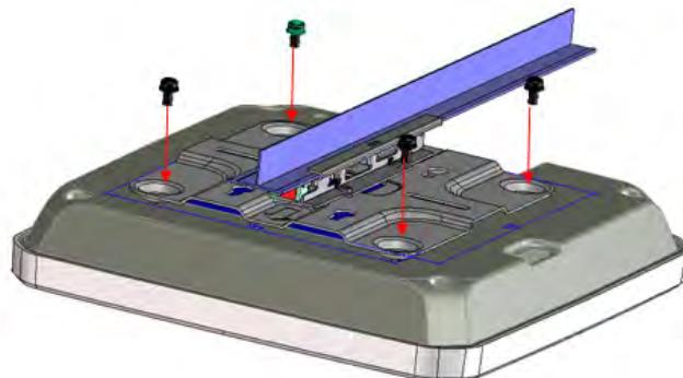
Note: Make sure the arrow on the main bracket is aligned so that it is pointing toward the top side of the Access Point.
