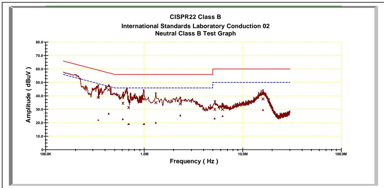
\* NOTE: During the test, the EMI receiver was set to Max. Hold then switch the EUT between Main antenna , Aux antenna Channel 1 , 4, 5, 8 ,9,12 of Normal Mode and Channel 1, 2, 3,4,5 of Turbo Mode to get the maximum reading of all these channels.
